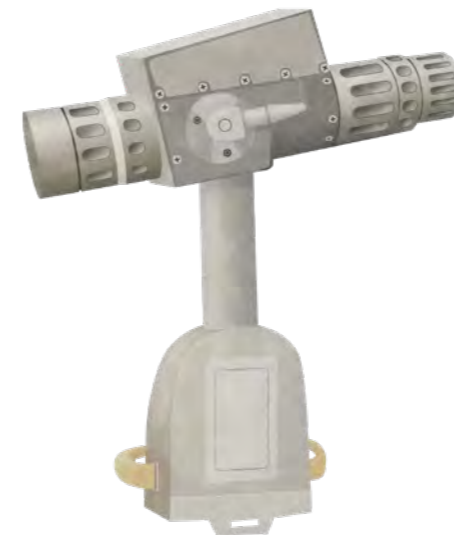
▲ Precise electric "screwdriver" that can be handled with thick gloves
